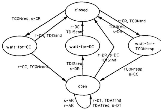
Fig. 7. State diagram of a transport protocol specification.
