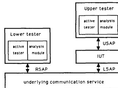
Fig. 3. Distributed test architecture.
