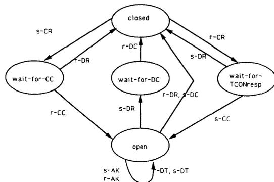
Fig. 8. State diagram of a reference specification for lower observer.
