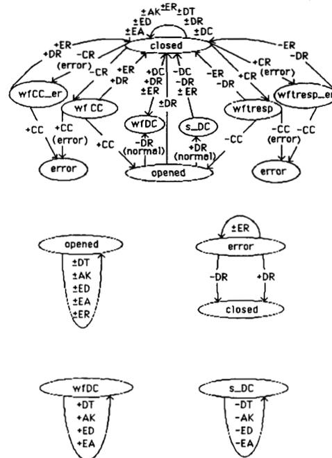
Fig. 10. State transition diagram for analysis module of transport arbiter.
