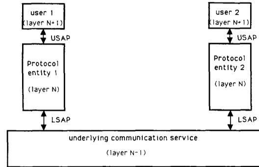
Fig. 1. Layered protocol architecture.
