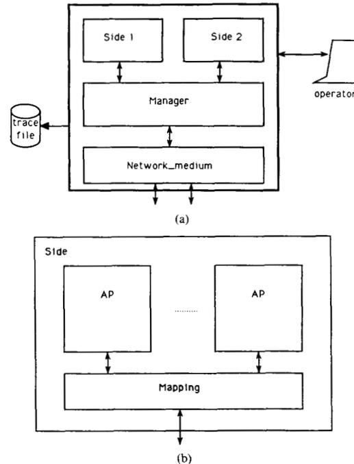
Fig. 9. (a) Estelle structure of arbiter. (b) Estelle structure for side module of arbiter.
