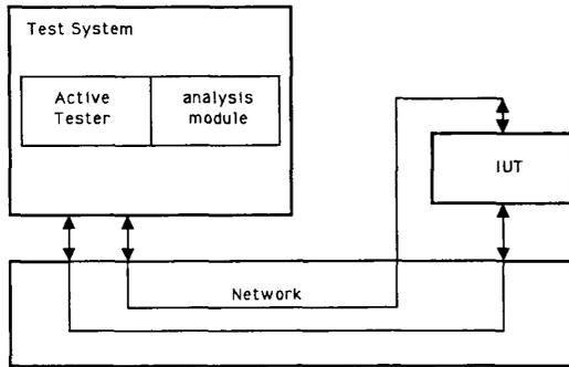
Fig. 4. "Ferry" or "astride" test architecture.
